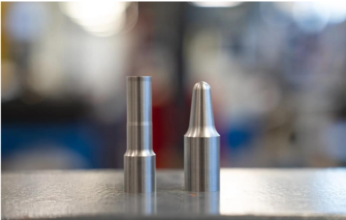
Close-up image of Foundation Alloy molybdenum-alloy forging die
