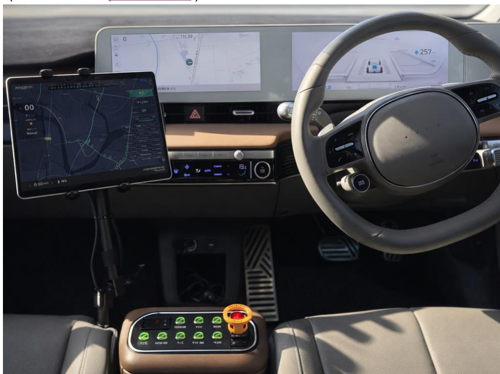
In-vehicle autonomous driving hardware: tablet terminal (left) and green buttons (bottom)
